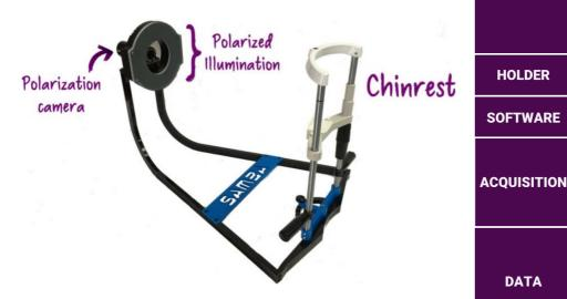
The SAMBA Face system has been specifically designed for the measurement of in-vivo skin gloss directly on the model body by separating the reflected light from the diffusion light. The system includes our SAMBA polarization camera, a polarized LED ring and an ajustable chinrest.
